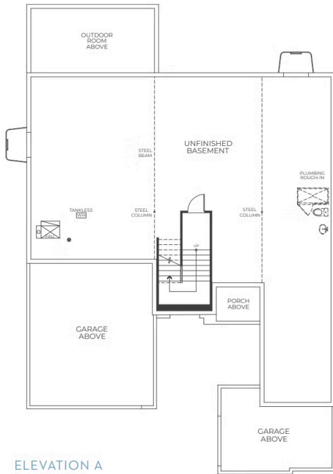
ELEVATION A BASEMENT
