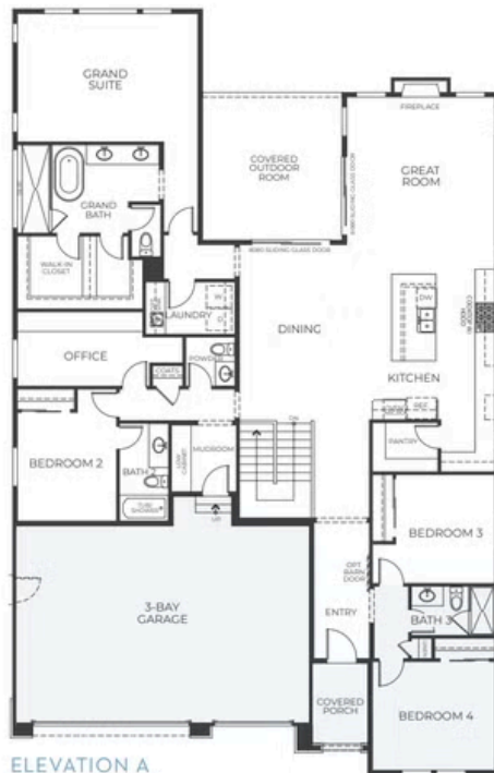
ELEVATION A FIRST FLOOR
